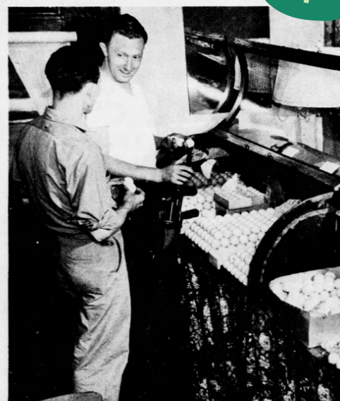
After the chemical wash and a water rinse, the balls are dried in the sun. The dried balls are then graded according to condition. Here Tyler is sorting them.
